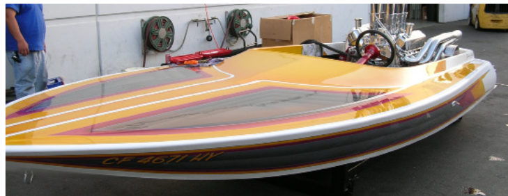
Tom Buckles' 18' Barron Sprint. Prime Marine built this from the bare hull on up, including floors, hardware and Pfaff 540 engine installation.
